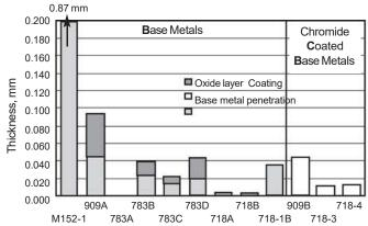
Figure 10- Measurements of metal affected by 1,009 hours of salt spray at 35°C in 5% NaCl. Testing was done as per ASTM B117-97. Trends indicate the resistance alloy 783 is far superior to other low CTE alloys and on par with alloy 718. Letters and numbers after the alloy show multiple samples.
