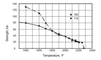
Figure 13- Gleeble fracture strength of alloys 783 and 718.
