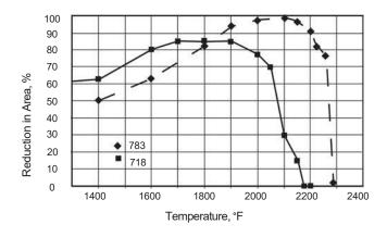
Figure 12- Gleeble hot ductility of alloys 783 and 718.
