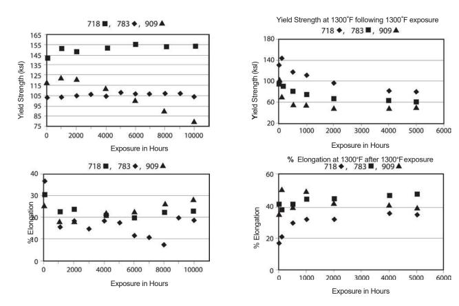
Figure 4 - High temperature tensile properties of INCONEL alloys 783, 718 and INCOLOY alloy 909 tested at 1200°F (649°C) following isothermal exposure at 1100°F (593°C).
