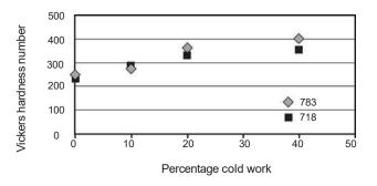
Figure 15- Work hardening characteristics of alloys 783 and 718.
